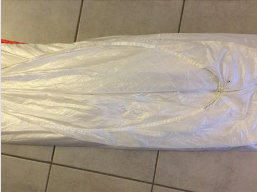
Position the rear tip on the top of the wound-up panels and open the gap. This special and easy packing method guarantees a much faster opening as the standard S-fold.
