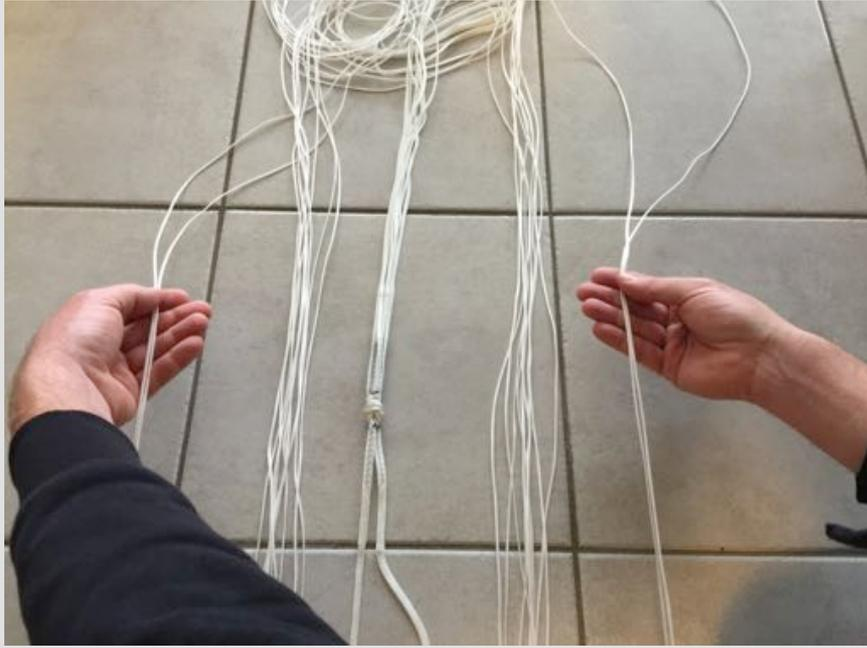
Follow the brake lines from the brake line riser to the canopy and check for twists.
