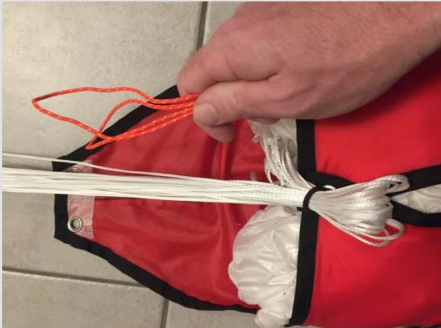
**CAUTION:** If the packing rope will not be removed, the parachute cannot open. This can cause malfunction, injuries or death!
