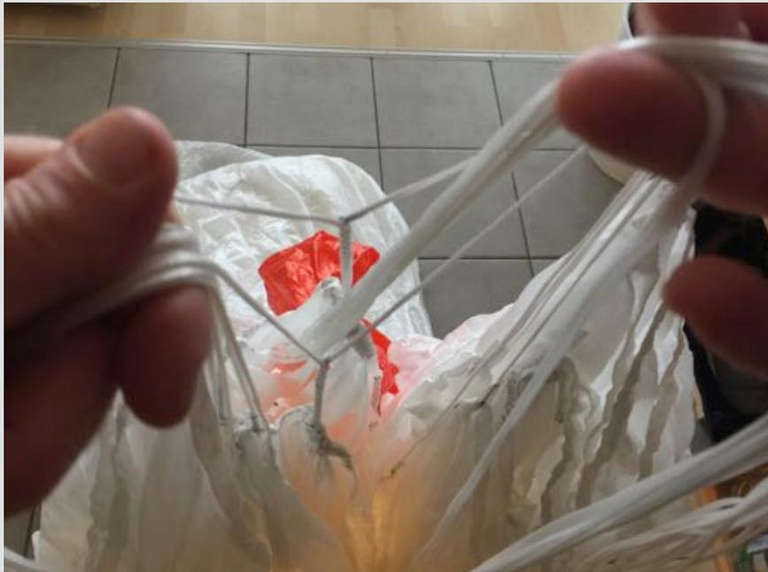
Continue and check that all centerlines are between the two front and two rear fork lines. **CAUTION: If the center lines are not between, there is a line over and the canopy is inside out.**
