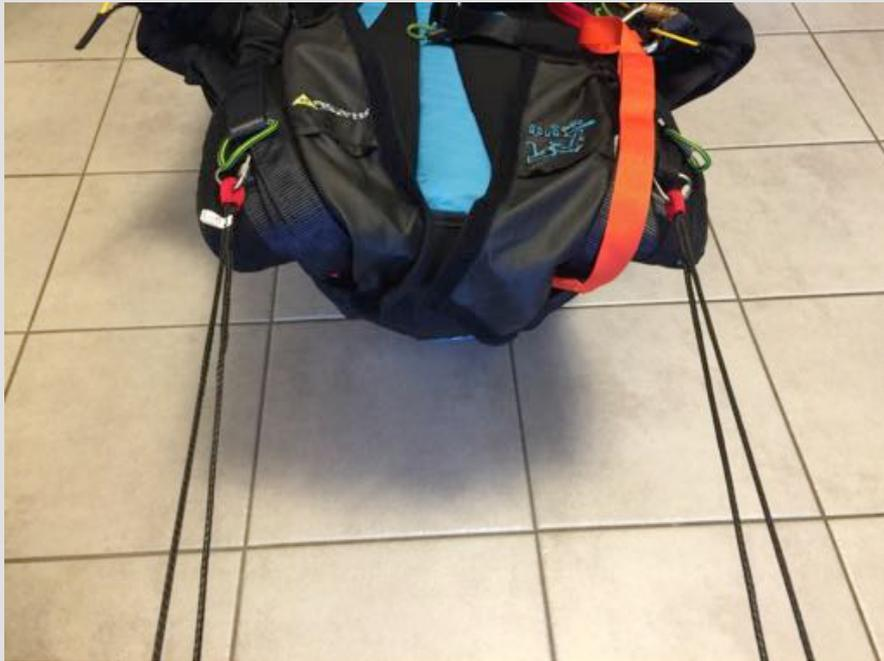
Install only approved connectors with at least 500 kg WLL (Work Limit Load). If you use Dyneema links, install them according to the instructions of the manufacturer.
