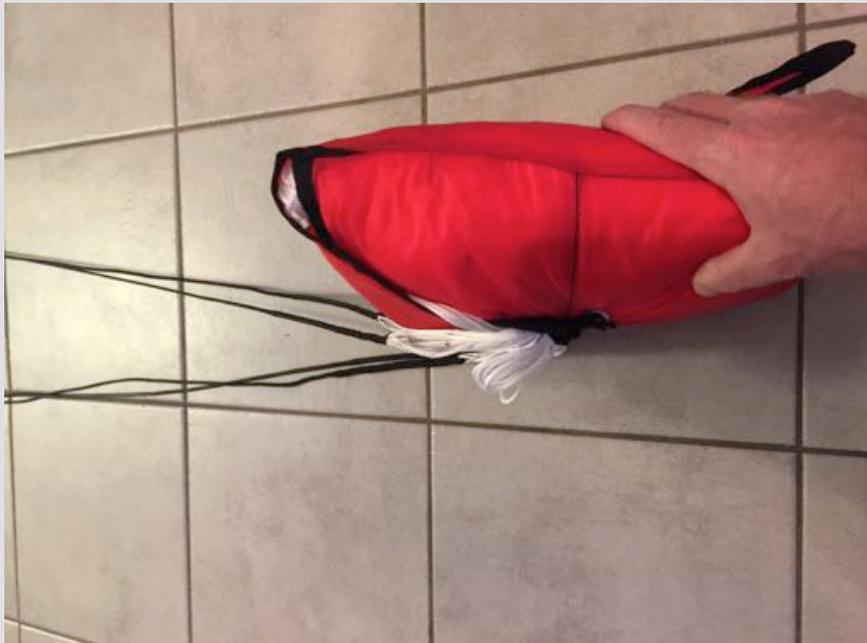
Twist the container 180° counterclockwise (direction of rotation, if you look in direction of the harness) and if the reserve parachute will be installed on the right side of the harness. Otherwise opposite.
