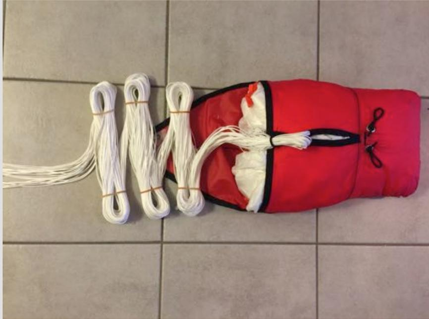
Position the lines according the picture and bundle the lines with three loops on each side of the bundle.
