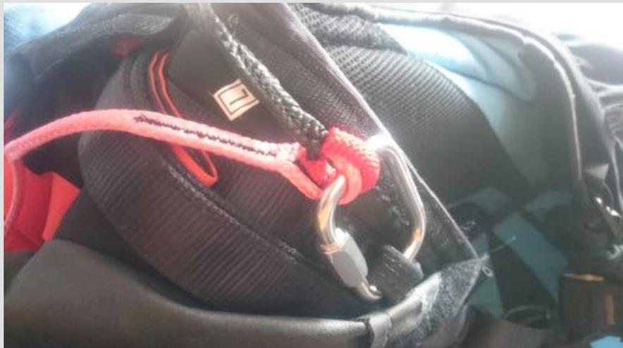
Connect riser and red safety connection with “L” or “Left” to left hand side (flight direction) of the harness. Connect RH riser and red safety connection to right side of reserve parachute attachment point of the harness. **Put both loops on each side into the shackle!**
