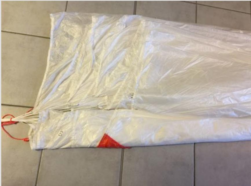
Fold panels two times at approx. 1/3 of depth in direction of the center. You may use packing clamps or weights.
