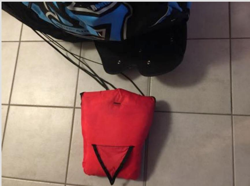
Move harness into upright position, install handle on the inside container. Pack risers (like V-lines) and container into the harness according the instruction of the harness manufacturer.
