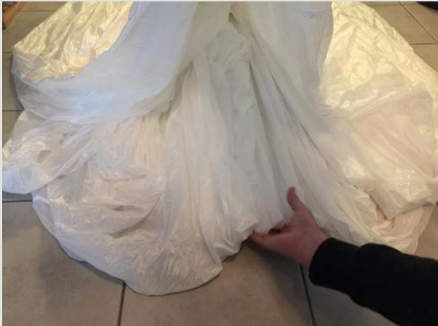
Pull back the material of the canopy around the contour of the parachute, so that outer and center lines are pre tensioned. This makes folding of the canopy easier.
