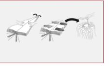
STEP 4: There are folding loops, nearly midway down the canopy where the panels were stitched. Pass a tie through these loops and stretch the parachute out.
