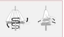
STEP 10: S-fold the left and the right side of the canopy one after the other in the direction to the centre of the chute. Keep the canopy neatly folded using sandbags.
