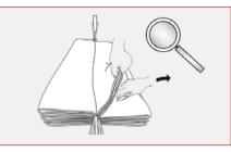
STEP 8: Lift the upper line to make sure the folds are neat along the whole length of the panels and that the wind channel is cleary right up to the apex of the canopy.
