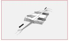
STEP 5: Separate the two outer lines (the outside lines on the riser) and lay them on the comb. Flake the canopy, starting with the lower panel on the right (panel 16), arranging it neatly.
