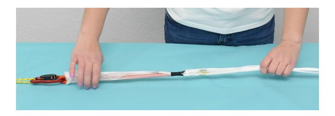
2. Find panel no.1, separate the panels and lines so that an equal amount lies on each side.
