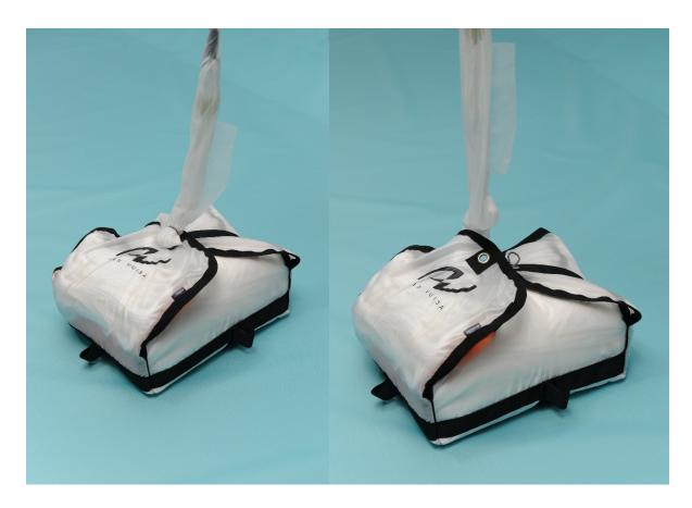
Now that we have properly packed our reserve parachute into the container, turn it on its back. On the back side you will see four attachment points with loops for connecting the rescue handle, which pulls the parachute from the rescue pocket of the harness.
