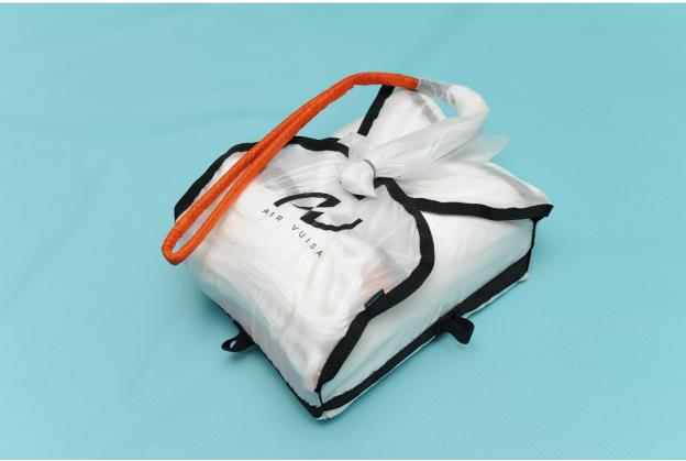
Note – Always perform a main loop release test, the loop should release and the container should open easily by its own if the reserve is packed properly!
