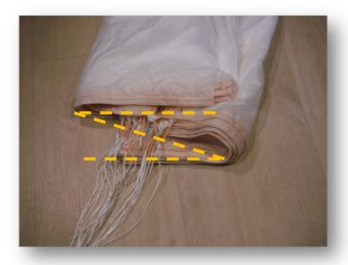
REMEMBER TO REMOVE ALL LINES OR RODS USED FOR FIXING PACKING LOOPS BEFORE FINISHING
