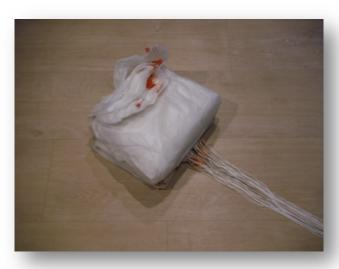
20. Install into the container upside down, the base edge needs to be on top!
