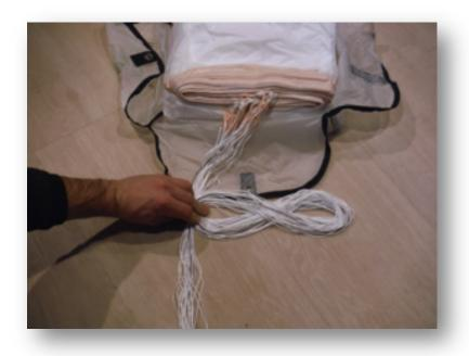
22. The width of the S-turns should be a bit shorter than the container side.
