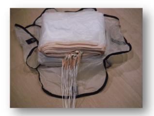
21. The lines should now be placed with narrow S-curves to a tower
