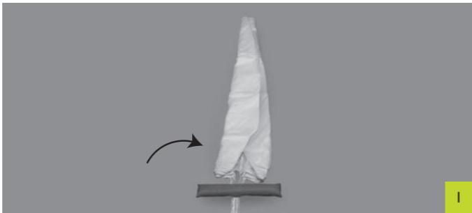
Fold the canopy in an accordion or "Z" shaped folds, so that it fits into the inner deployment bag. If possible, adjust the folds so that those at skirt level are slightly shorter and those at the top of the canopy are slightly longer. The CIRES rescue fits well if there are 4 folds. (Image J and K)
