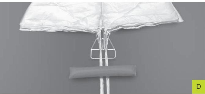
Follow the outer suspension line to find the centre panels and begin the folding process. ([Image E](#))
