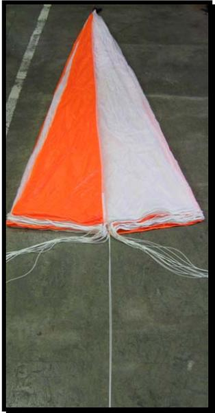
Keep the skirt even and suspension lines separated each side of the apex lines.
