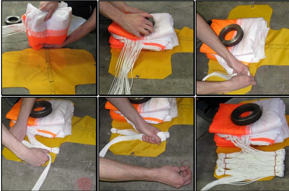
Carefully lift the lines on top of the folded canopy and bring the 2 flaps together feeding the elastic closing loop of flap 1 through the eyelet of flap 2 opposite.
