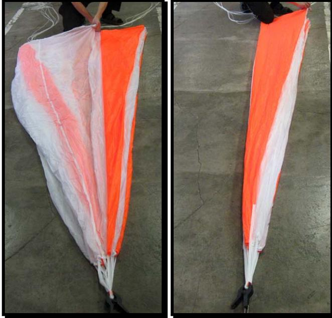
Next fold each panel one by one to the other side of the suspension lines. Again check each panel for damage and make sure it is flat and without creases.
