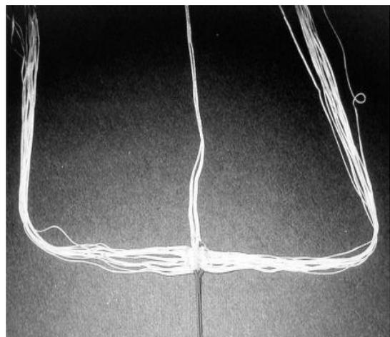
Please make sure that the middle lines are in the middle and the other lines to the side. There must not be any tangles or knots in the lines.
