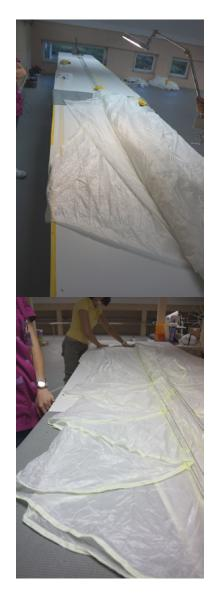
The first two panels when folded form a triangle. The other panels are laid flat and tightened. The last panel (Tip of Rogallo) is to be folded in a triangular shape.
