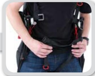
Fasten the leg/chest strap by placing the male buckles through the female buckles on each side
