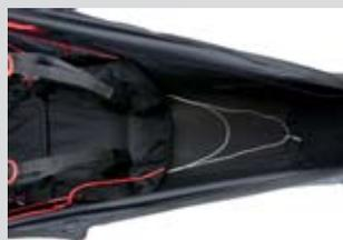
Ensure the speed system lines are of equal length. Check that the lines are not too short as this may inadvertently activate the speed system when under tension in the air. Double check on the ground before flying.
