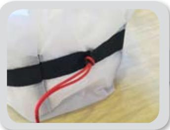
Attach the reserve handle to the deployment bag using a larks foot through the loop.
