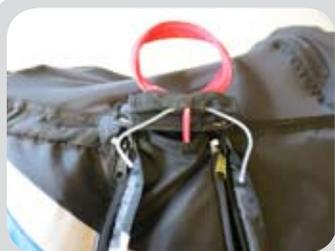
The container can now be closed by running the both zips forward, all the way to the eyelets.
