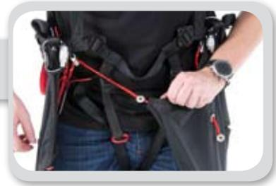
The Cockpit is zipped to the top of the pod. In the air it rests over the top of the chest strap. The supplied elastic chord is optional. It can be placed over your head and allows the cockpit to maintain a good position during launch
