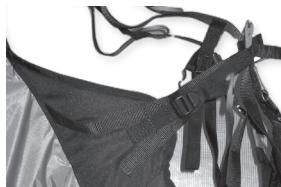
**Lumber support** – Adjust so that it is comfortable for your style of flying. Fully tightened will give an upright position, for a more reclined (supine) position release the lumber support straps.
