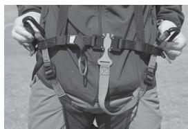
**Chest strap** – The maximum setting is 44cm which is ideal for most pilots and is the distance Ozone recommends. It is possible to reduce further by tightening the strap in the air.
