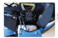
Pay attention to the bidles. Do not allow them to become entangled, they should remain neatly in place to the left hand side of the parachute when inserting.
