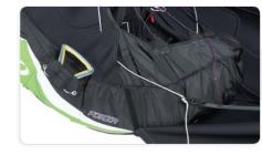
Ensure that the lines run cleanly between the pulleys and pass on the outside of all structural webbing straps. Double-check the lines have not inadvertently wraped around any of the structural webbing straps. Attach the speed bar with a Bowline knot and repeat the proceedure on the other side.
