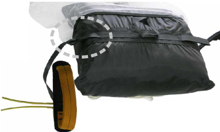
Enclosed handle have to be attached asymmetrically at the lateral loop of the rescue-system's inner container.
