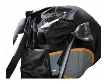
Store the bridle of the rescue-system in a kind of S-shape into the container of the harness.
