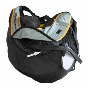
Open the channel of the bridle and take out this V-shaped bridle of the harness.
