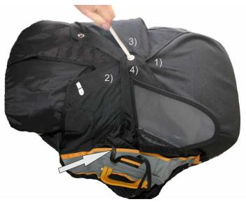
Close the container with packing cords. First the rear flaps have to be closed in the right order (1,2,3,4). The connection of the handle runs between the flaps 2) und 4). You have to take care that the connection of the handle is not hindered in any way!
