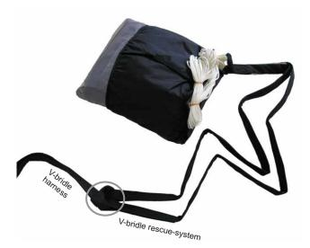
The bridle of the rescue-system has to be connected to the single end of the V-bridle of the harness. If also the rescue-system has a V-shaped bridle (as you can see in the picture), you have to take care that both ends of the V-bridle of the rescue-system are connected to the single end of the harness' V-bridle.
