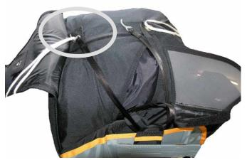
...and fix it immediately with one of the pins. Then remove the frontal packing cord!!
