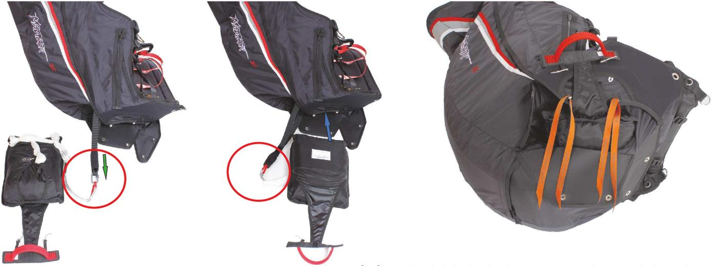
1. Connect the rescue bridle with the harness bridle by looping the bridles or with a quick link (strength > 2400 daN) and fix the connection to prevent slipping (for example by a neopren sleeve).
