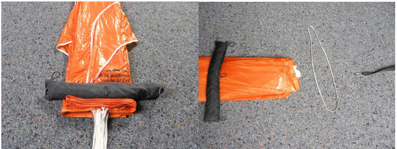
1. Fold the parachute like a "S" on the width of the container, pull out the Ram-Air-pockets a little bit to the side (if the parachute is equipped with Ram-Air-pockets).
