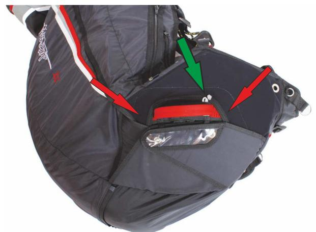
6. Remove all packing cords! Close pin covers and place the handle in the neoprene pockets (red arrow), secure handle with a 2 daN seal threat (green arrow).
