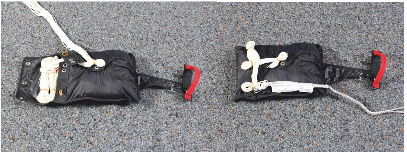
4. Close the deployment bag with the lines. First the right flap with the upper and lower flap. Depending of the rescue system size the inner or outer grommets can be used to adjust the deployment bag volume.
