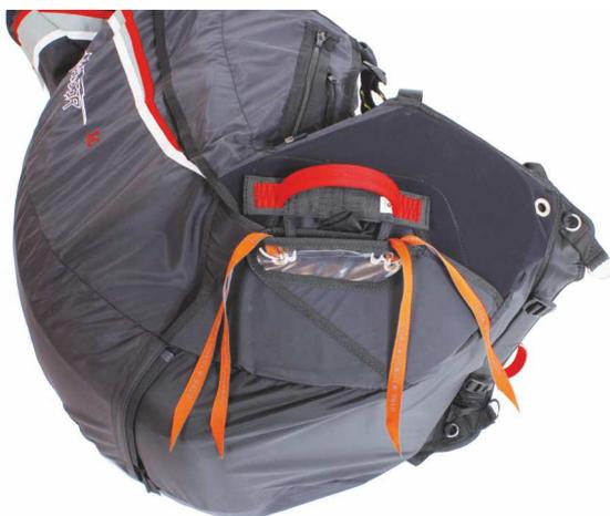
5. Close third container flap with packing cords. Put the pins through the loops.
