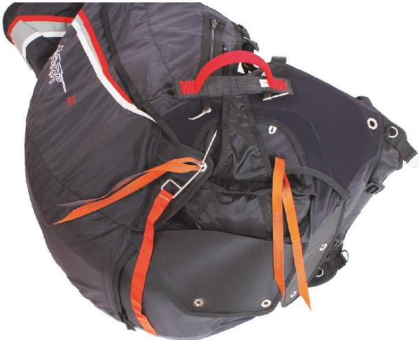
3. Close the first container flap by using the loops with the help of the packing cords. Place the handle-deployment bag connection in between the 2 grommets.
