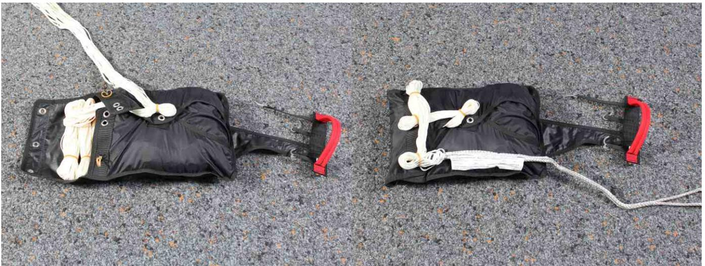
4. Close the container with the lines. First the right flap with the upper and lower flap. Depending of the rescue system size the inner or outer grommets can be used to adjust the container volume.
