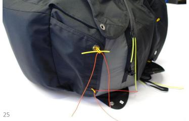
Lead the assist lines through the loops of the #6 and #6a flaps. Connect the # 6 and #6a flaps and lock them with temporary pin as shown on the left. Lead the assist lines through metal grommets in the # 5 flaps and lock them with temporary pins.
