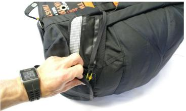
Close the pins cover with a velcro strap and place the strap of the release handle in a tunnel on the #2 flap.
