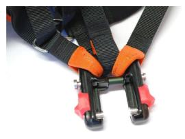
After clipping riser of the paraglider to the Quick Out carabiner, move the locks of the buttons in order to avoid unintentional release.
