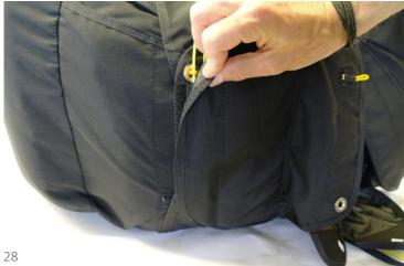
Close the pins' cover with a velcro strap and place the strap of the release handle in a tunnel on the #4 flap.
