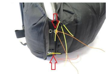
Lead the assist lines through metal grommets of the # 1 flap and lock them with temporary pins.
