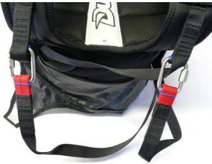
Tighten the nuts of the quicklinks with a wrench.
