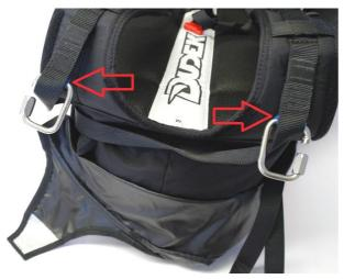
Fix the additional V-riser to the attachment points on the shoulder straps with two C6 lockable quicklinks as shown on the pictures.
