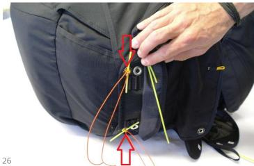
Lead the assist lines through metal grommets of the # 4 flap and lock them with temporary pins.
