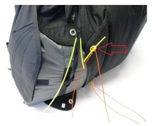
Lead the assist lines through the loops of the #3 and #3a flaps. Connect the # 3 and #3a flaps and lock them with temporary pin as shown on the left. Lead the assist lines through metal grommets in the # 2 flaps and lock them with temporary pins.
