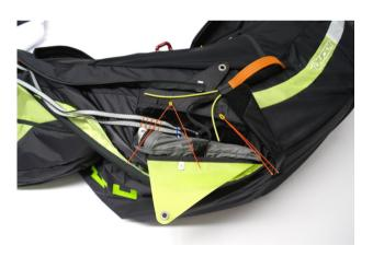
Lead the assist line through the metal eyelet of the #1 flap and secure yellow loop with the longer pin. Put the end of the pin into its pouch. Gently remove the assist line.
