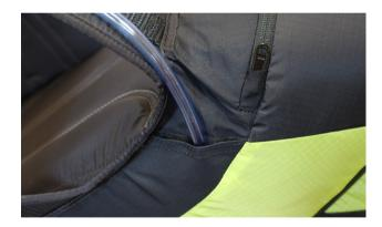
I The rear part of the harness including the back pocket fills with the air during flight. That's why the opening is closed with a velcro. Close it carefully at all times, so that the spillout for the back pocket is minimized.
