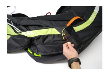
Secure it with the shorter pin. Put the pin through the holes of the #2 flap as pictured beside. Gently remove the asisting line.
