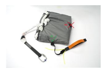
Connect both ends of the V-riser with the riser of the rescue chute with a Maillon Rapide C6 quicklink.
