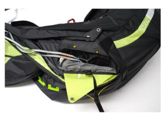
Place the end of the release handle in a dedicated pouch and fix it to the side of the harness with a velcro.
