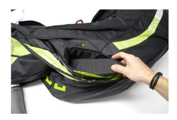
Put the rescue chute in the container, so that the release handle remains on top.
