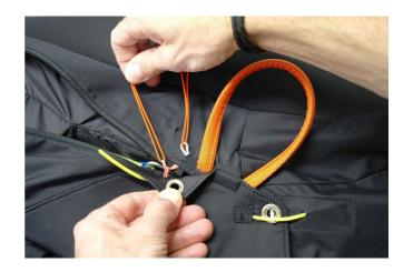
With an assist line put the white loop through the higher red one as shown.
