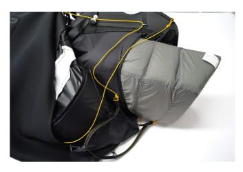
The airfoam pad fills the space between pilot's back and the rescue chute container. It improves the seating comfort while offering additional protection.
