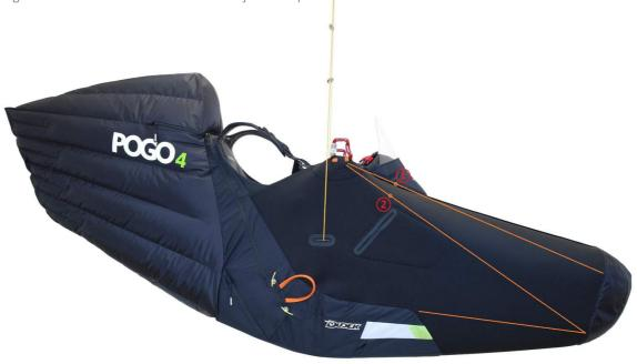
Length of the left upper line can be adjusted after earlier tensioning of the pods right side. It can be done by moving red ball #3 until desired effect is reached. The right side of the pod is closed by inserting ball #4 and #5 in the loops of the safety strap #6. The left side is closed and adjusted by the #7 buckle. This part of the pod is integrated with the cockpit.
