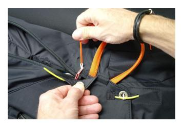
Lead the white loop through the metal eyelet and secure it with a pin.
