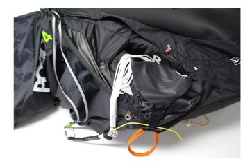
Put the loose parts of the bag inside, so as to cover the line loops closing the bag.
