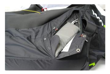
The harness is equipped with a pin to close the empty part of the container. Close the container as described above.
