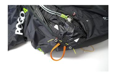
Using the assist line lead the loop through the metal eyelet and block it with a pin.
