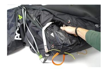
Place the lines and riser of the rescue chute in the container as shown beside.
