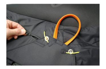
Close the V-riser tunnel by moving the slider towards the upper part of the harness.
