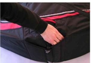
See that #1 flaps inside the container are not folded and properly guard the rescue chute.
