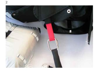
Connect the rescue chute riser to the V-strap of the harness with locked quicklink.
