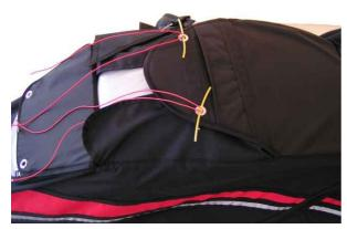
Lead assist lines through #3 flap, with optional use of temporary pins.
