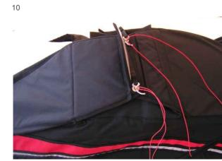
Close the container with regular pins and remove assist lines. Put them under the pins first, so that container loops are not damaged by friction.
