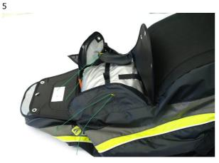
Lead the assist lines through the loops of the #1 flaps.
