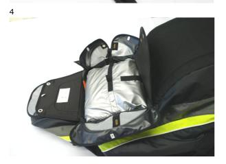
Put the rescue chute in the container with suspension lines facing downward. Both the lines and the riser of the canopy must be stoved in the rear part of the container. The container is a bit deeper there.
