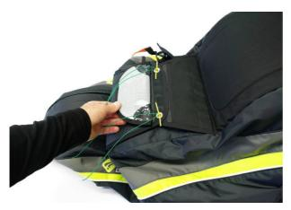
Lead the assist lines through the loops of the #3 flaps, with optional use of temporary pins.
