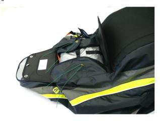
Flap #1 is divided in two. Put the riser attaching handle to the bag between both parts of the flap. Lead the assist line through the fragment equipped with a metal loop.
