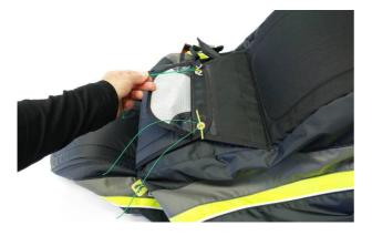
Close the container with regular pins and remove assist lines. Put them under the pins first as shown below, so that container loops are not damaged by friction.
