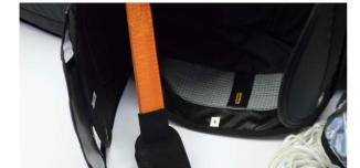
After locking the quicklink secure the straps by applying neoprene cover to keep them in place.
