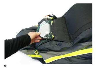
Lead the assist lines through the loops of the #3 flap, with optional use of temporary pins.
