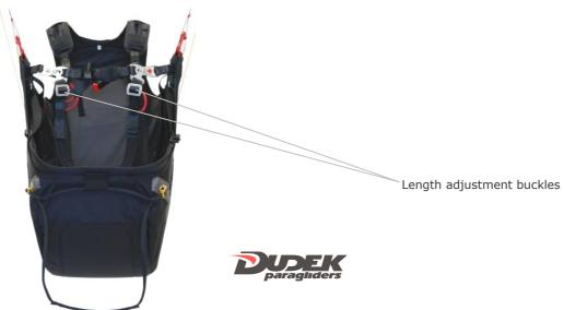
In order to avoid falling out of the harness it is imperative to check before each launch if the chest and legs straps are closed. Not closing the straps is extremely dangerous and is a known reason of fatal accidents!
