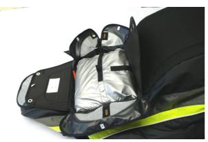
Put the rescue chute in the container with suspension lines facing downward. The lines and riser of the canopy must be stoved in the rear part of the container. It is a bit deeper there.
