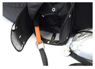
Connect the rescue chute riser to the V-strap of the harness with locked quicklink Maillon Rapide C6 or C7. It should be locked with a wrench so that a chance opening is impossible.
