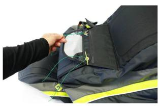
Close the container with regular pins and remove the assist lines. Put them under the pins first, so that container loops are not damaged by friction as shown on the picture.
