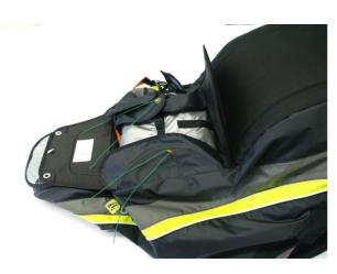
Flap #1 is divided in two. Place the strap connecting release handle to the rescue chute between both parts of the flap. Lead the assist line through the fragment equipped with metal loop.
