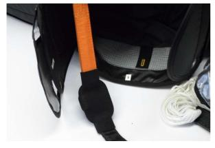
After locking the quicklink safeguard the straps by applying neoprene cover to keep them in place.
