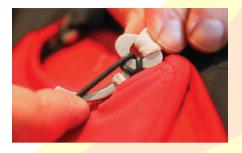
IPull the rubber O-ring around the pin to secure the pins.
