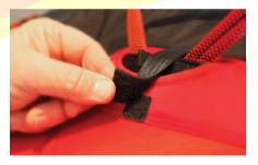
Attach the Velcro retaining strap.
