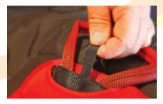
Verify there is enough slack in the strap connecting the handle to the reserve so that the pins will be pulled first.
