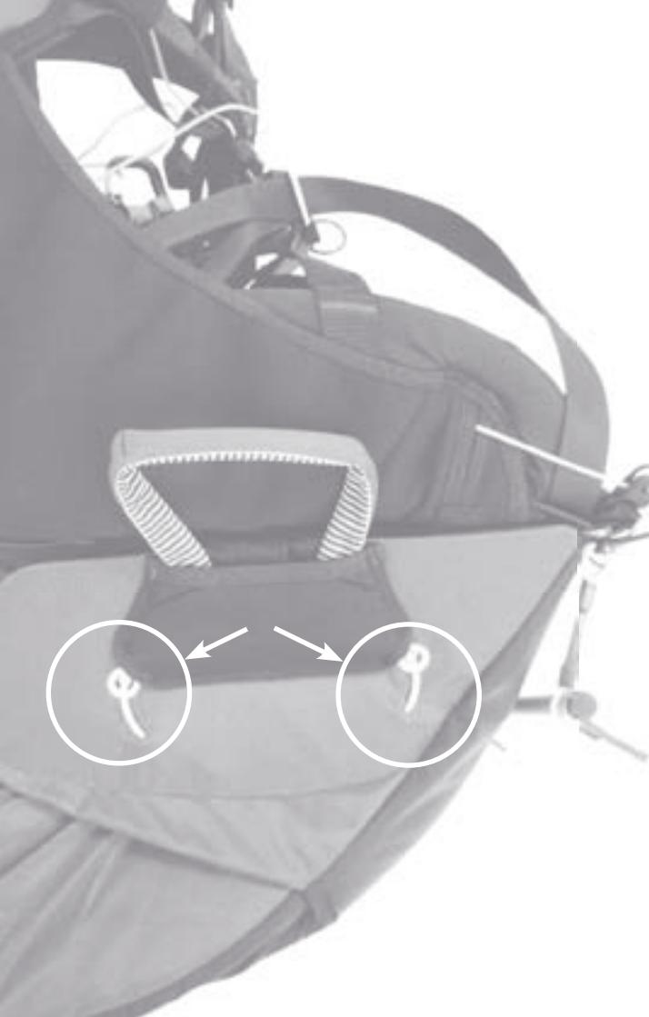
The deployment handle is held on the right side of the harness in the neoprene pocket provided. The two pieces of yellow cable on the deployment handle are led through the openings in the neoprene pocket, through the closure loops and into the 'buttonholes'. The handle will then lie next to the harness, is well visible and easy to reach. Always check that the two yellow cables are routed cleanly, so that a correct parachute release can be guaranteed.
