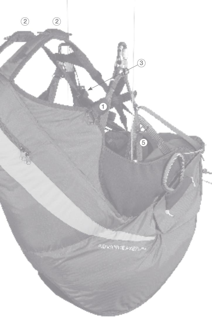
ments, and these are marked with white sewing on the straps for the back and legs. To start a full adjustment open the shoulder, chest and seatboard straps fully. The pictures in this handbook show the various adjustment possibilities.
